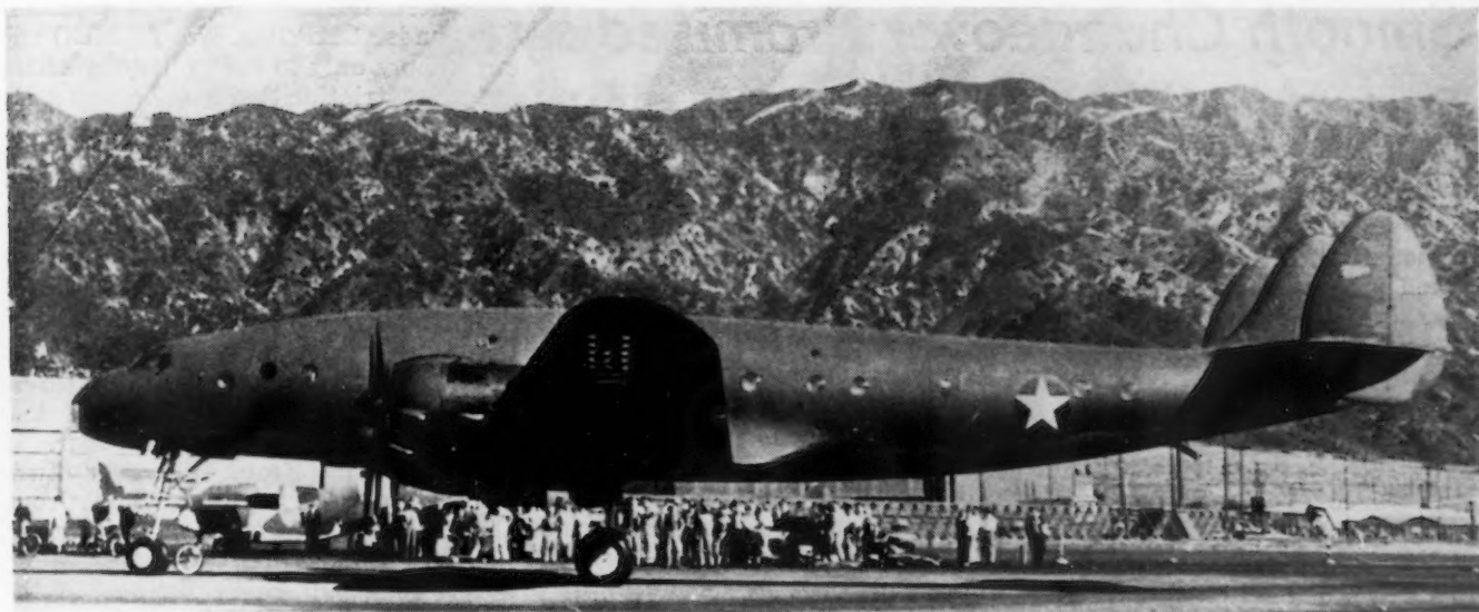
LARGEST, FASTEST TRANSPORT: Capable of carrying men and large quantities of equipment over long range, the Lockheed "Constellation" is reputed to be the largest, fastest and most powerful land-based transport plane in flight. The mighty ship is shown prior to her initial flight from the Lockheed Air Terminal in Burbank. Its four 2,000-horsepower Wright engines are mounted in an airframe of new aerodynamic efficiency. At cruising speed, at about half power, the Constellation is approximately 100 miles an hour faster than standard air-cargo or airline ships of today. The Constellation is able to cruise through thin air at 20,000 feet and yet maintain air density of an 8,000-ft. level in the pressurized cabin. In case of need, the Constellation can rise comfortably to 35,000 ft.
